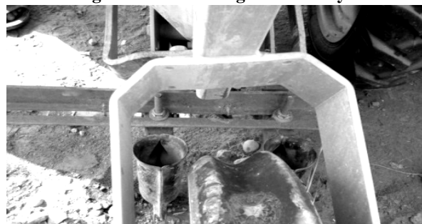
Fig. 6: After ridging rearward curve furrow opener
