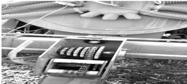
Fig. 7: Gear box for change grain plate speeds.
