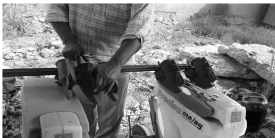
Fig. 5: A rearward curve furrow opener
