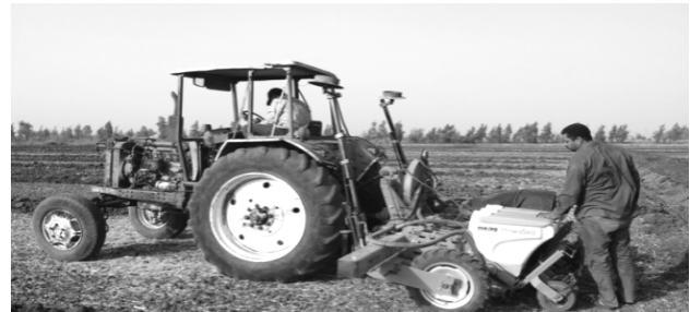
Fig.8: Vacuum precision planter.
